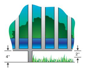
Where the barrier is mounted on top of the pool structure, the maximum vertical clearance between the top of the pool structure and the bottom of the barrier shall be 4".
