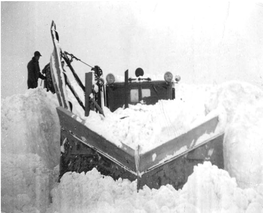
1947 – V Plow with Wing on North Road
